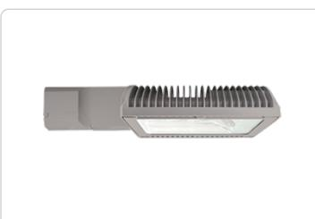
LED roadway lighting that's easy to buy. Free trial program and leasing options make it easy to get started with LED. Specification-grade optics deliver efficient, clean, uniform light distributions at a reasonable cost. Optics are factory installed and meet IES Lateral Distribution Type III. LROAD™ 78W replaces 250W metal halide roadway fixtures.
